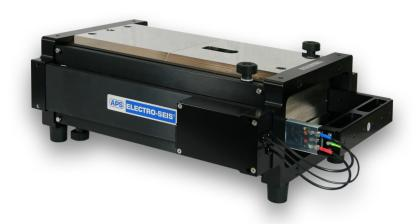
The **APS 400 ELECTRO-SEIS**® shaker is a longstroke, electrodynamic force generator specifically designed to be used alone or in arrays for studying dynamic response characteristics of various structures. It finds use in modal excitation of complex structures, particularly when low frequencies are required. Furthermore it can be used for low frequency vibration testing of components and assemblies.
